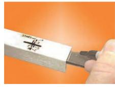
3. Scribe a line through the dot. The line should extend across the width of the Tension-Finder tool. Then go back to step 4 on page 1.
