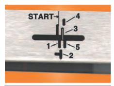
Step 7: Determine the required slot for your drive from Table 1. Tighten the belt until the line has moved to the designated slot. (In this photo, the line is in Slot 3.)
