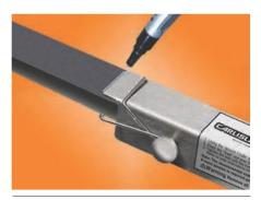
Step 6: Scribe a line at the spring end of the Tension-Finder tool. Use this line as a reference point in case the spring slips off the belt.
